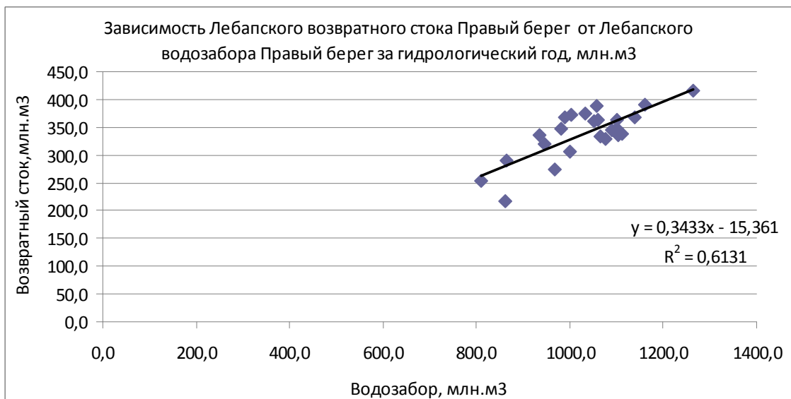
Fig.24. Relationship between the Lebab return flow, right bank, and the Lebab water intake, right bank, in hydrologic year, mcm
