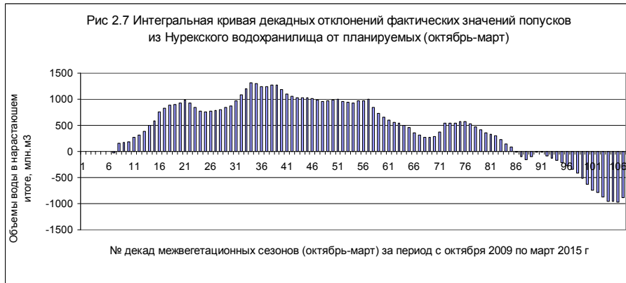
Fig.2.7. Cumulative curve of ten-day differences between actual and planned water releases from Nurek reservoir (October-March)
