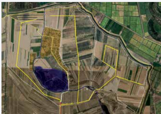
Concept for three pump-buried pipe systems covering 1090 ha pumping from a reservoir (tank) in tail of Secondary Canal, K18, Makhtalar Scheme
