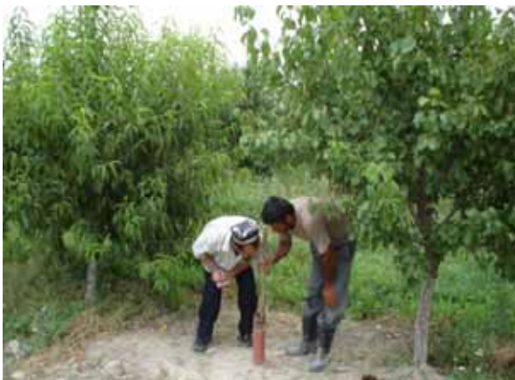
Measuring a watertable depth
