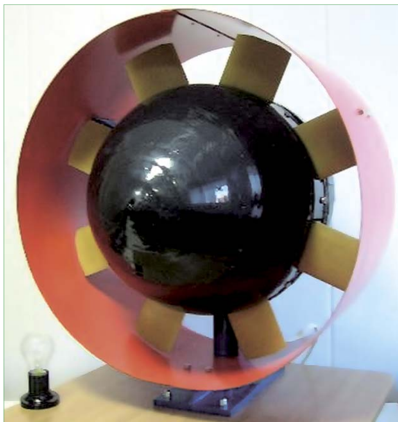
Fig. 2. MicroHPP Turbogenerator “Aquatron – 300”
