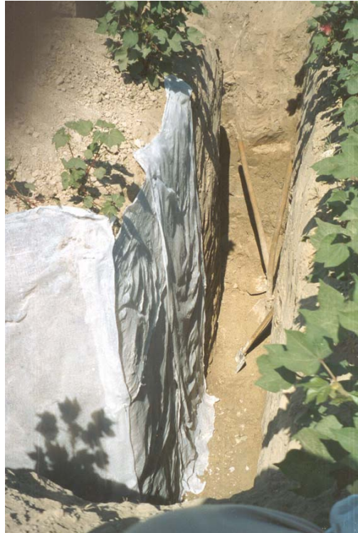
Fig. 2. Preparation of the soil monolith to avoid lateral water fluxes.
