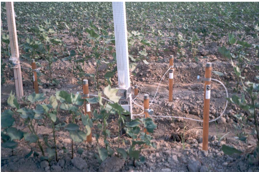
Fig. 3. Two sets of tensiometers and neutron access tubes in a monolith, Fergana.
