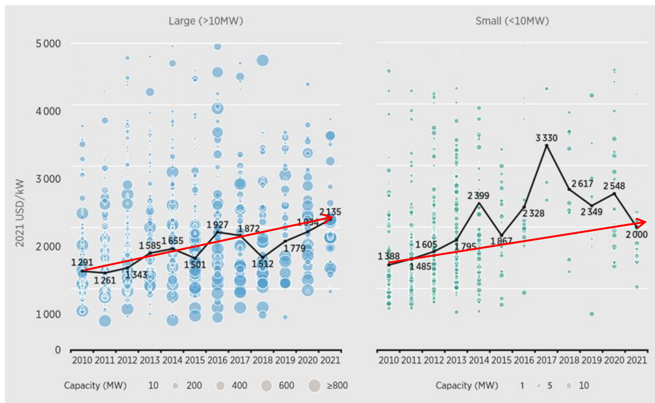
Figure 6.3 Total installed costs for small and large hydropower projects and the global weighted average, 2010-2021
