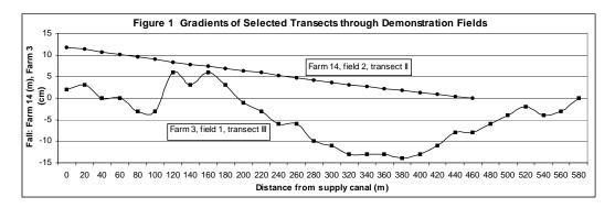
Relative height of the land surface was measured at points on a 20m x 20m grid. Based on the vertical sections along transects, decisions were made on the sub-division of the field by temporary field canals.
