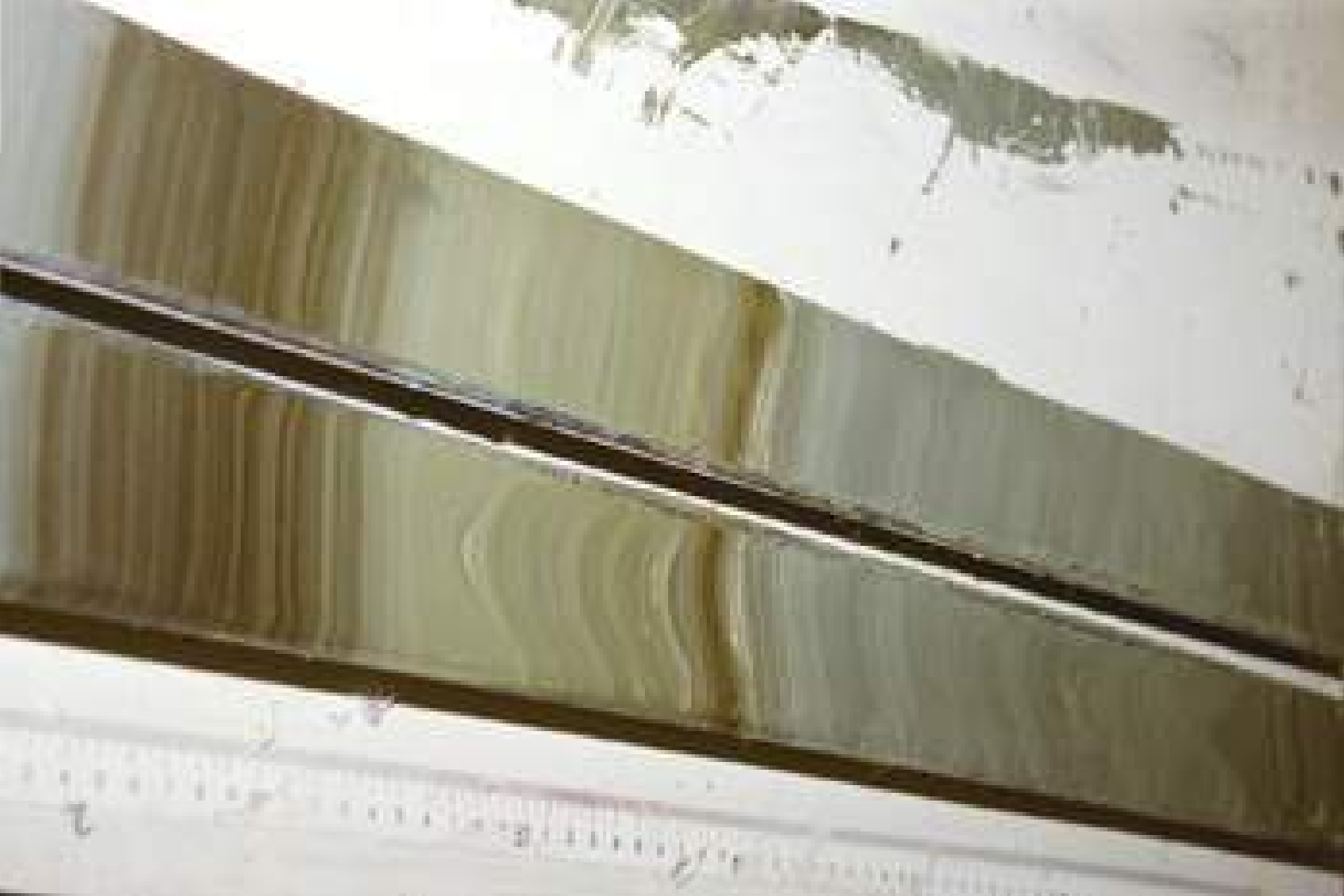
Cut cores. Layers of deposits are neatly visible.
