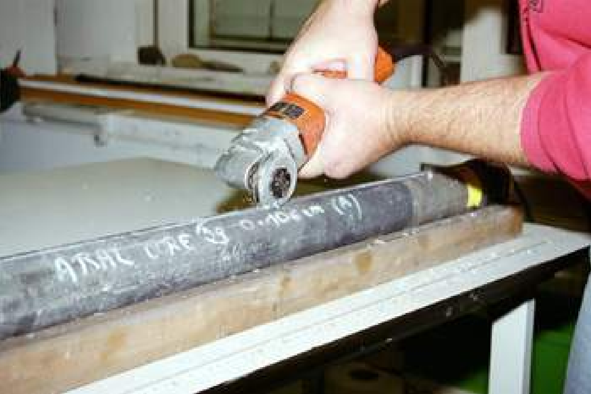
Cutting plastic tube containing core of bottom sediments
