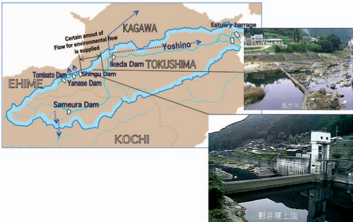
Fig. 5.11.13 Arrangement of facilities after completion of the Tomisato Dam
