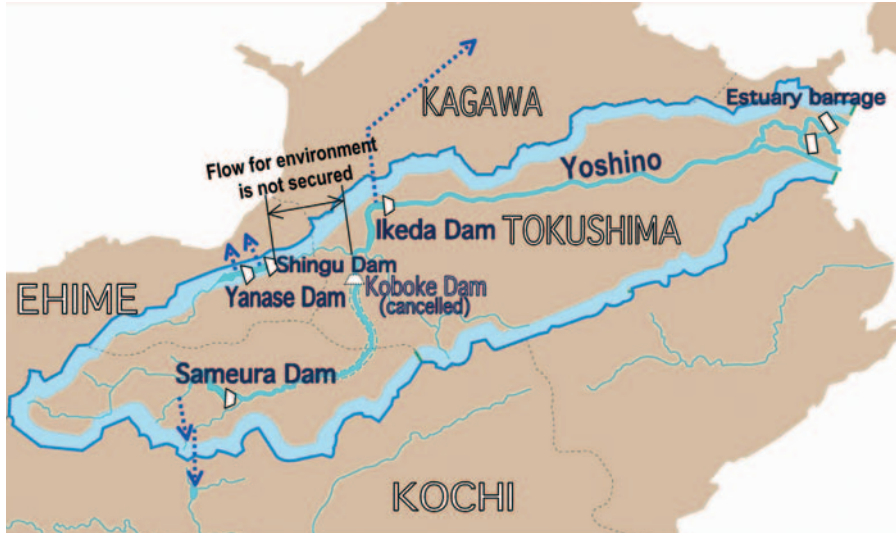
Fig. 5.11.12 Arrangement of facilities in 1975 (after completion of YCDP)
