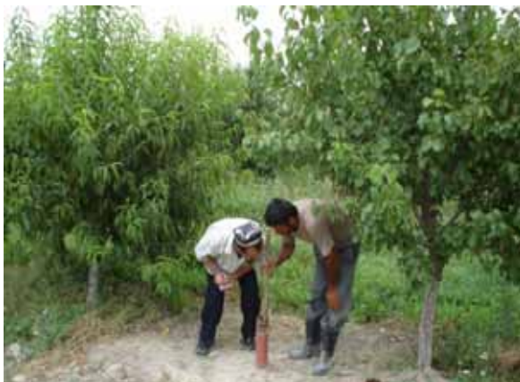
Measuring a watertable depth
