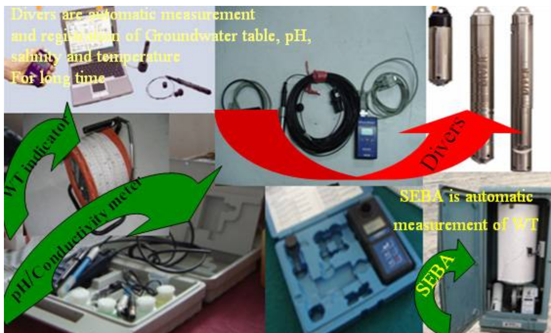
Figure 2 Water Table and Physical parameters measurement devices
