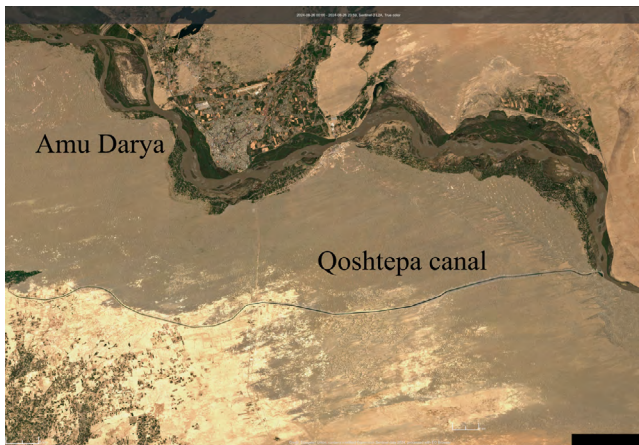
Figure 7. Sentinel-2 satellite image showing first phase of construction, with work starting in Kaldar District in Balkh Province, bordering Tajikistan. This section of the canal is also partly filled by groundwater seeping into it during the excavation due to higher groundwater levels close to Amu Darya.
